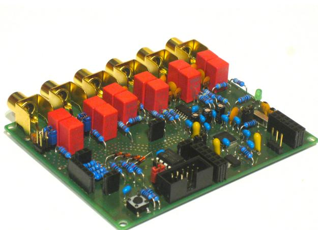
Figure 3: Completely assembled freeDSP module (V 0.4).
