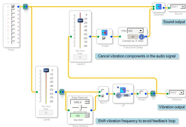
Figure 8: Simplified program patch in SigmaStudio, showing one approach for vibration generation by frequency shifting the violin sound (bottom path). Additionally, the vibration crosstalk in the audio output is canceled actively using an inverter and a fractional delay (top path).
