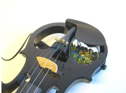
Figure 7: Vibrotactile feedback for an electric violin using a small electro-dynamic on the backside of the chin rest. The freeDSP was integrated in the free space below.
