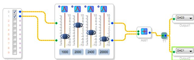
Figure 4: A simple example patch in SigmaStudio.
