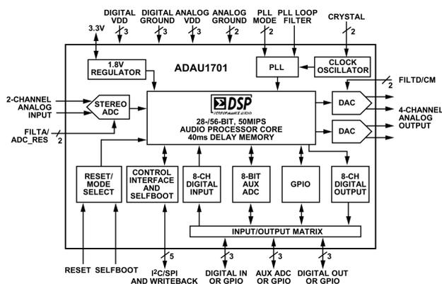
Figure 1: Functional block diagram of the ADAU1701 from Analog Devices [2].
