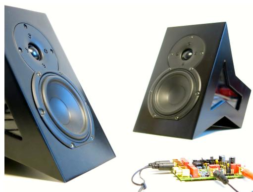
Figure 5: Small active loudspeaker prototypes with digital crossover, loudspeaker protection and bass enhancement algorithms. An early version of the freeDSP can be seen in the foreground.
