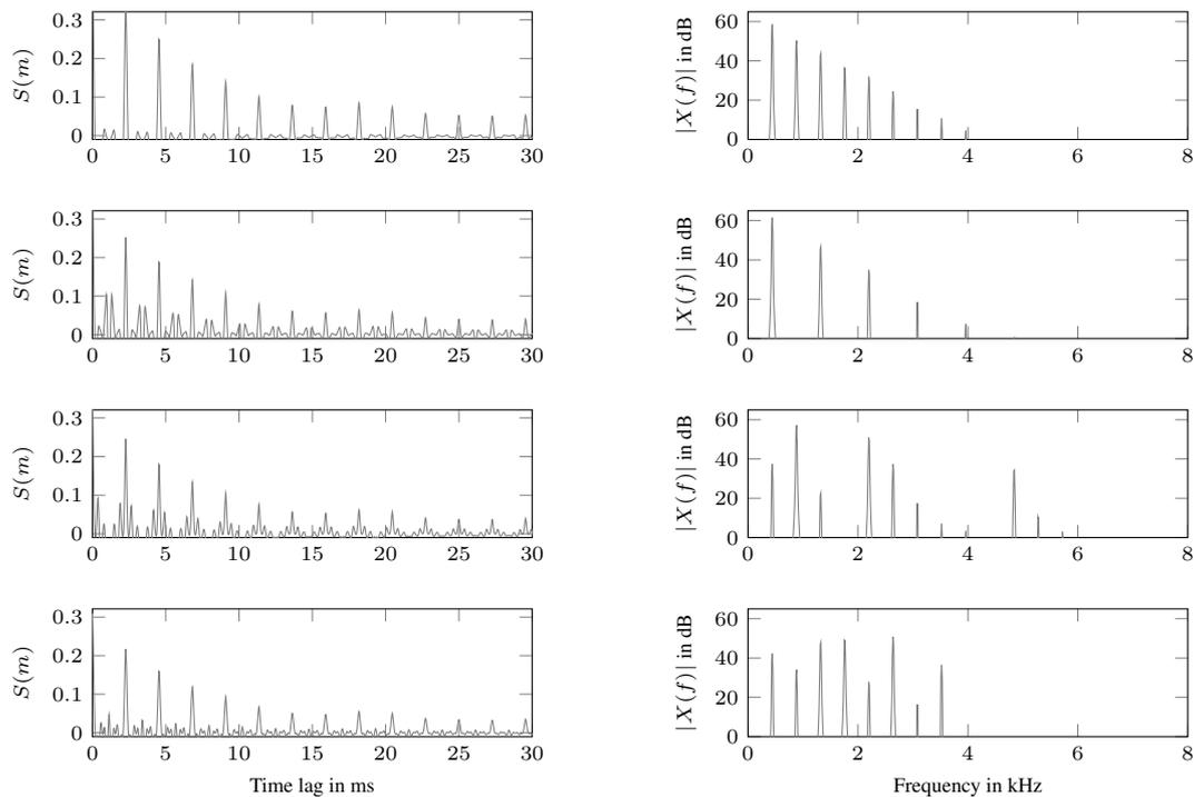
Figure 2: Outputs of the summary autocorrelation function (SACF) for input signals with different spectral envelopes. Fundamental frequency of all signals is 440 Hz which corresponds to a period of 2.27 ms.
